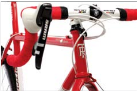
Ritchey WCS Cross fork and headset with integrated cable hanger included.
