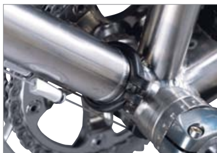
Patented compression coupling system joins front and rear triangles near the bottom bracket shell. Quick-Disconnect cable adaptors included.
